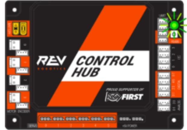
1. The one BIG advantage the Control hub has over the Expansion hub is that you don't need RC phone which gives more space on your robot.
